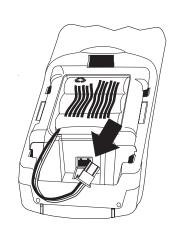
4. Place the battery pack inside the battery compartment, and slide the battery cover back on.
